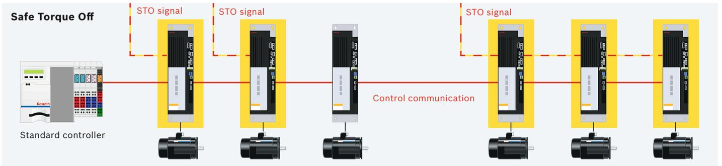
**Safe Torque Off: For safe interruption of applied torque**
