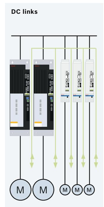
is reduced. This improves network compatibility and allows smaller components to be used without compromising machine performance.
