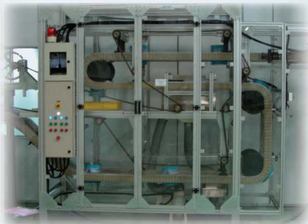
Gripper conveyor with blower attached to remove dust from products.
