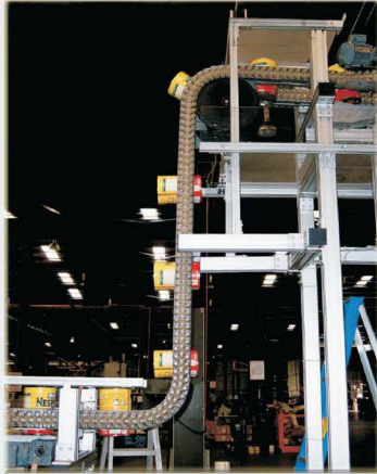
S-Type Gripper Conveyor to elevate empty tin can
