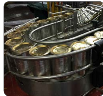
Thermoplastic Chain with Stainless Steel Beam Conveyor
