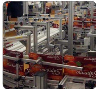
Thermoplastic Chain with Aluminum Beam Conveyor
