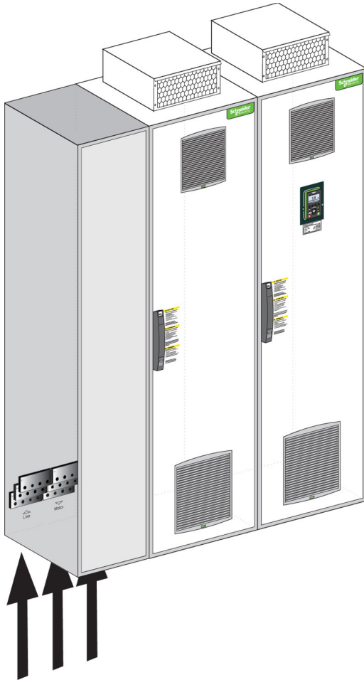
Additional enclosure allowing cabling from the bottom
