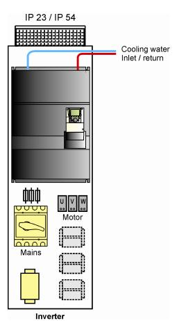
Liquid cooling of electrical and mechanical units is already best-proven in the area of plastics machines. Due to their robust cooling system, the ATV 61Q & ATV 71Q frequency inverters can be particularly integrated into existing cooling concepts.
