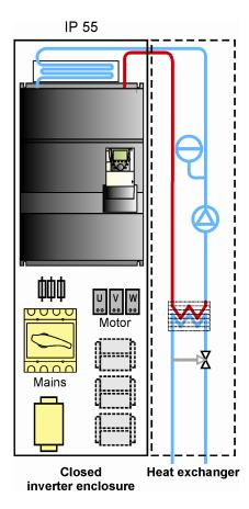
Enclosures in protection degree IP55 or higher, closed containers or also pressure-resistant encapsulation require a complete heat abstraction of the whole electrical drive unit. Therefore 100 % of the losses must be dissipated by the cooling water. This can be done easily with an additional air/water heat exchanger. Thereby the monitored fans in the inverter provide the required air circulation inside the enclosure.
