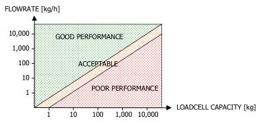
The performance is very dependent on the weighing system repeatability. It is desirable to aim for as high a repeatability as possible. With care, it is possible to achieve weighing repeatability of 1 part in 10,000 to 1 part in 100,000.
