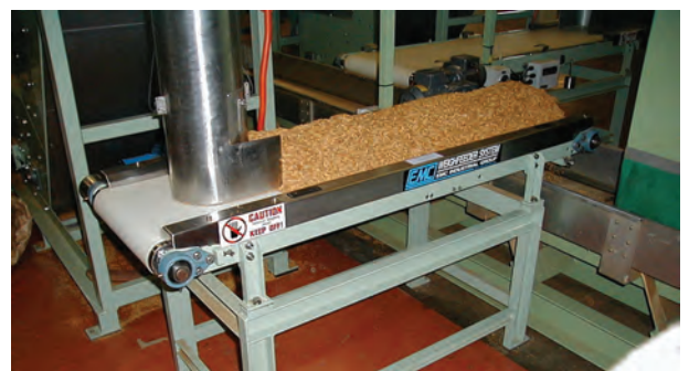
Weigh Feeder installed at tobacco plant
