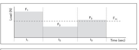
$$F_{m} = \sqrt[3]{\left|F_{1}\right|^{3} \cdot \frac{\left|n_{1}\right|}{n_{m}} \cdot \frac{t_{1}}{t_{ges}}} + \left|F_{2}\right|^{3} \cdot \frac{\left|n_{2}\right|}{n_{m}} \cdot \frac{t_{2}}{t_{ges}} + ... + \left|F_{n}\right|^{3} \cdot \frac{\left|n_{n}\right|}{n_{m}} \cdot \frac{t_{n}}{t_{ges}}}$$
