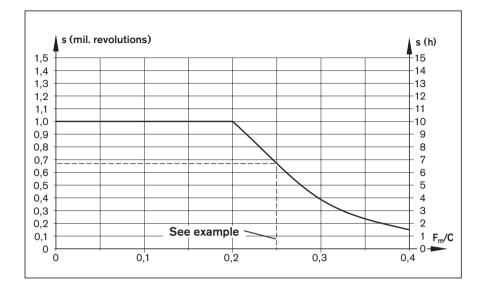
Conversion of lubrication interval s from millions of revolutions to kilometers:
