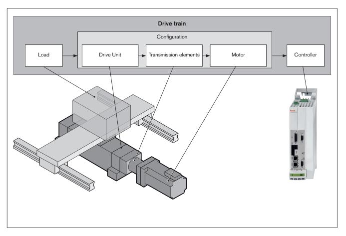
Correct dimensioning and assessment for an application requires structured consideration of the entire drive train. The basic element of the drive train is the configuration, consisting of the Drive Unit, the transmission element (coupling or timing belt side drive) and the motor, that can be ordered from the catalog.
