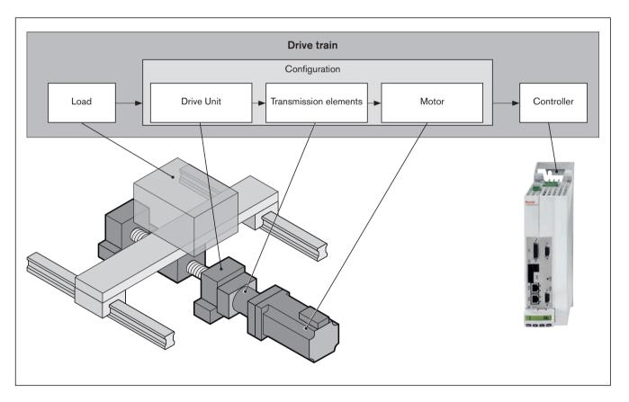
Correct dimensioning and assessment for an application requires structured consideration of the entire drive train. The basic element of the drive train is the configuration comprising the Drive Unit, the transmission element (coupling or timing belt side drive) and the motor, which can be ordered in this constellation as per the catalog.
