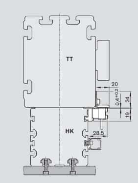
Proximity switches with attachments / cable duct
