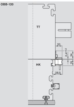
Proximity switches with attachments / cable duct
