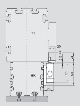
Mechanical switches with attachments
